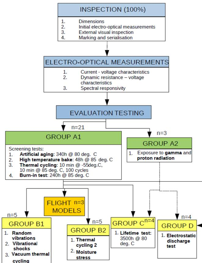
Fig. 2: Evaluation test program of the PVI-5 detectors dedicated for the EXOMARS space mission.
