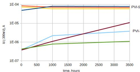
Fig. 5: The drift of the dark current of the PVI-3 and PVI-5 detectors during lifetime test.
