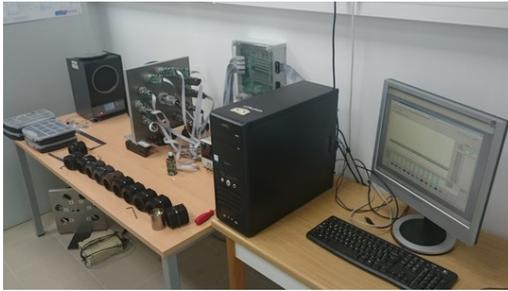
Fig. 9: The measurement set-up for acquiring the signal from 11 4-element PV-3TE-5 detectors.
