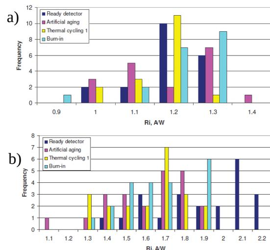
Fig. 4: Histogram of  $R_i(0)$  distribution after the screening tests for a) PVI-3 and b) PVI-5 photodiodes.
