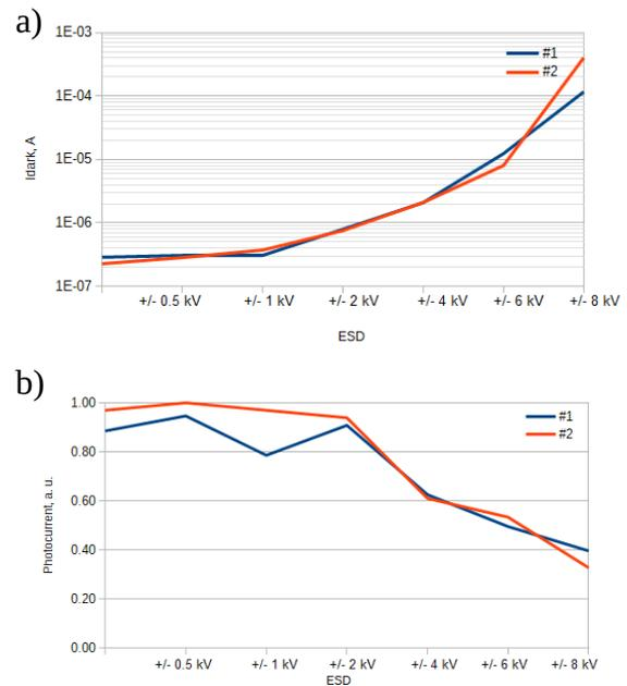
Fig. 6: The dark current and photocurrent at 3  $\mu\text{m}$  of 2 PVI-3 as a function of the ESD value.
