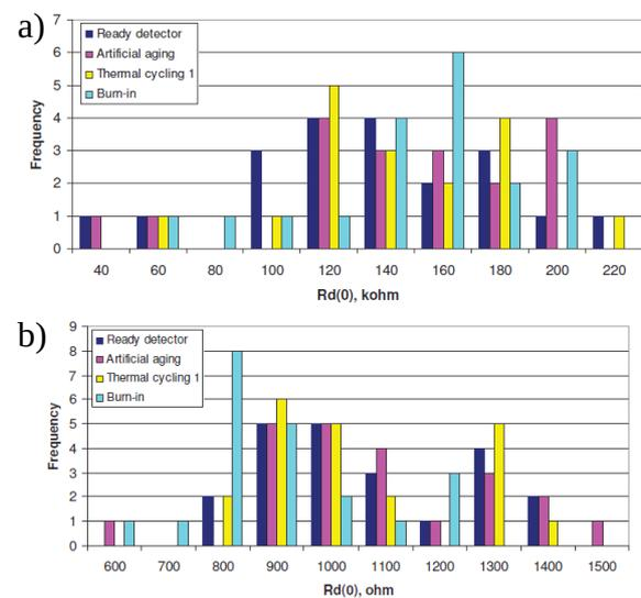
Fig. 3: Histogram of  $R_d(0)$  distribution after the screening tests for a) PVI-3 and b) PVI-5 photodiodes.
