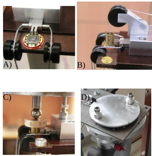
Fig. 8: The photograph of the experimental stands for application of A) transversal force, B) transversal force and longitudinal pulling, C) transversal force and longitudinal pushing, D) application of centrifugal acceleration.
