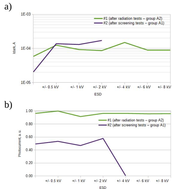
Fig. 7: The dark current and photocurrent at 5  $\mu\text{m}$  of 2 PVI-5 as a function of the ESD value. Prior to the ESD test, detector #1 had been subjected to the radiation tests, detector #2 to the screening tests.
