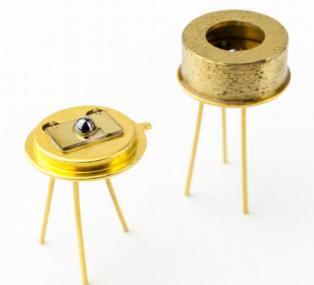
Fig. 1: PVI detector in TO39-based package.
